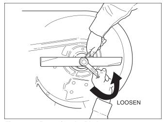
Figure 25. Removing the Blade
